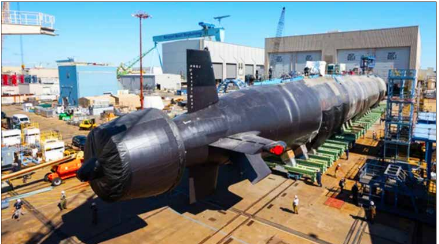
Using a transfer car system, the Virginia -class submarine Montana (SSN-794) was successfully transferred from a construction facility to a floating drydock at Newport News Shipbuilding division in preparation for its launch. (Photo by Matt Hildreth/HII.)
