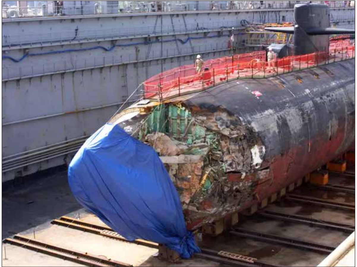
The damage to USS San Francisco after her underwater collision. (U.S. Navy photo.)
